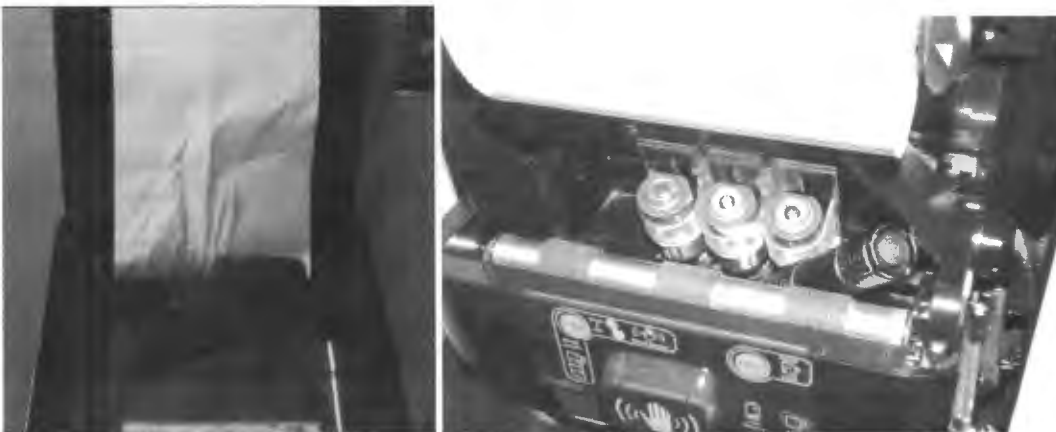
At left, charred end of paper towel roll exposed to fire; at right intact batteries inside dispenser.
